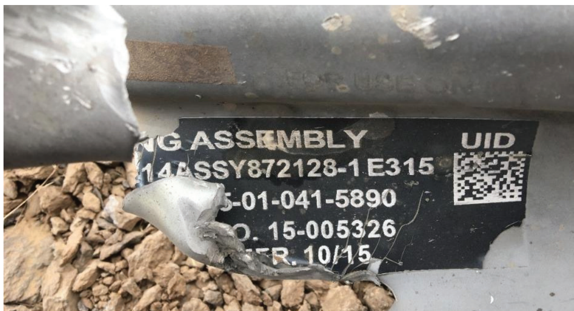
Remnant of a wing assembly that is mounted on a US-made GBU-12 Paveway II laser-guided 500-pound bomb found at the Arhab water drilling site, Sanaa governorate, where at least 31 civilians were killed in an airstrike on September 10, 2016. According to the manufacturing date as well as the national stock number, this wing assembly was produced by Raytheon Company, a US defense contractor, in October 2015.
