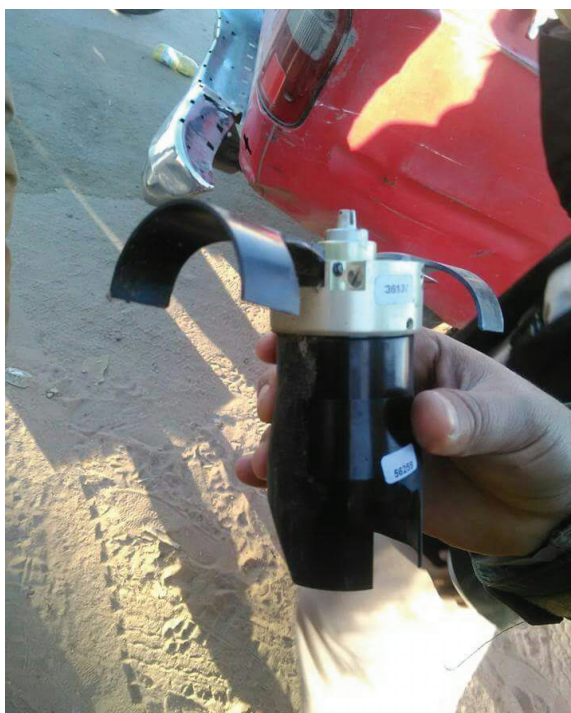
Submunition of an ASTROS II cluster munition rocket found in Saada City on December 7, 2016. Bahrain and Saudi Arabia have purchased ASTROS rockets from Brazil, where they are manufactured by Avibrás Indústria Aeroespacial SA. Each cluster munition rocket contains up to 65 submunitions. Unexploded submunitions are extremely volatile and can explode on contact: they should never be touched or handled. © 2016 Private
